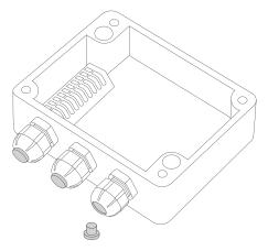
3. Pull the soil moisture sensor through the cable gland. You can connect one, two or three soil moisture sensors as required.
