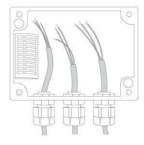
4. The soil moisture sensors should be connected according to the markings on the PCB, the sensor placed in CH1 should be inserted into the connectors marked "1" on the PCB, etc.
