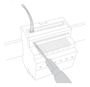
3. Screw the power supply wires to the device regardless of polarity (6 - 30 V DC, 5 - 21 V AC).
