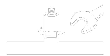
6. Plug and screw the 4-pin electrical connector into the sensor.
