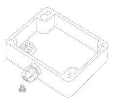
3. Pass the cable through the cable gland.
