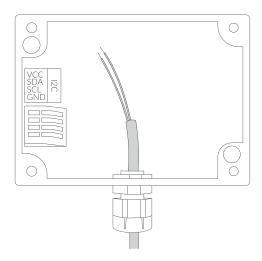
4. Press the spring contact and insert the appropriate wire into the corresponding slot in the connector:
