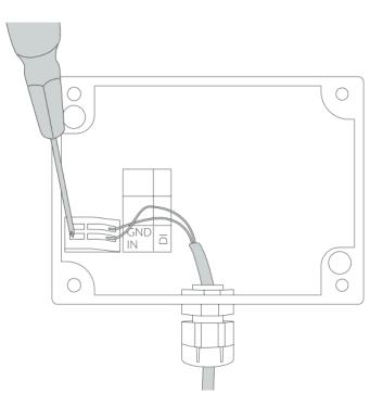
Figure 12 Connecting input cable instructions.
