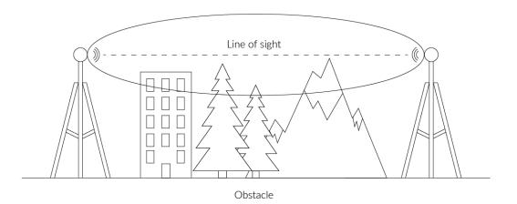
Figure 15 Fresnel zone where communication between two antennas can occur.
