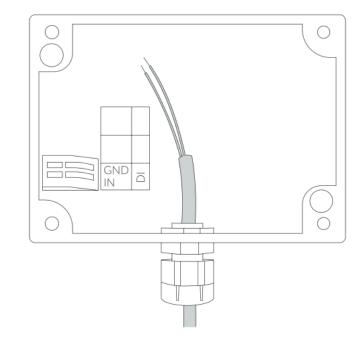
Figure 11 Input cable passing through the cable gland instructions.
